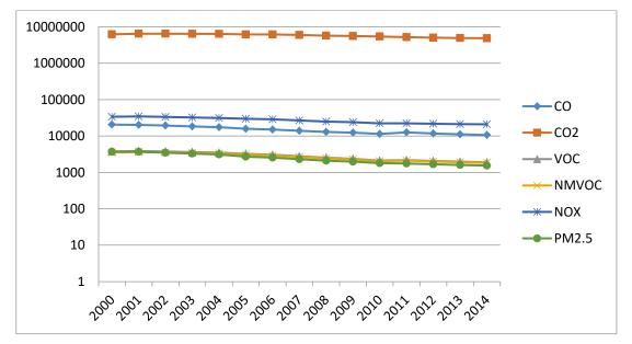
Figure 5. Light Commercial Vehicles - annual emissions in tonnes (logarithmic scale).
