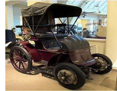
In 1899 an electric car was built, which Porsche presented as "Semper Vivus" ("Always alive") at the Paris World Exposition in 1900. (Hightspeed 50km/h, reach 50 km)
