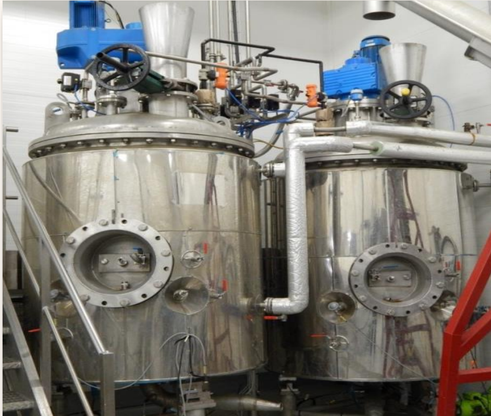
Bioreactors for enzymatic degradation
