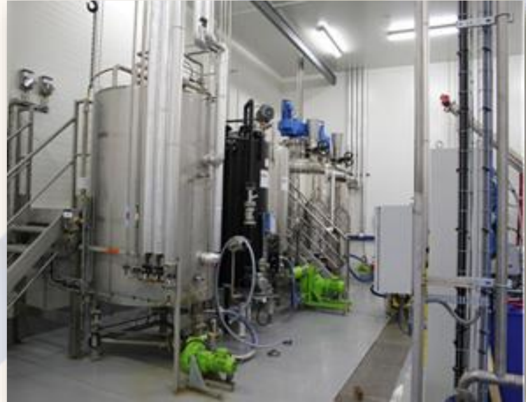
Bioreactors for enzymatic degradation
