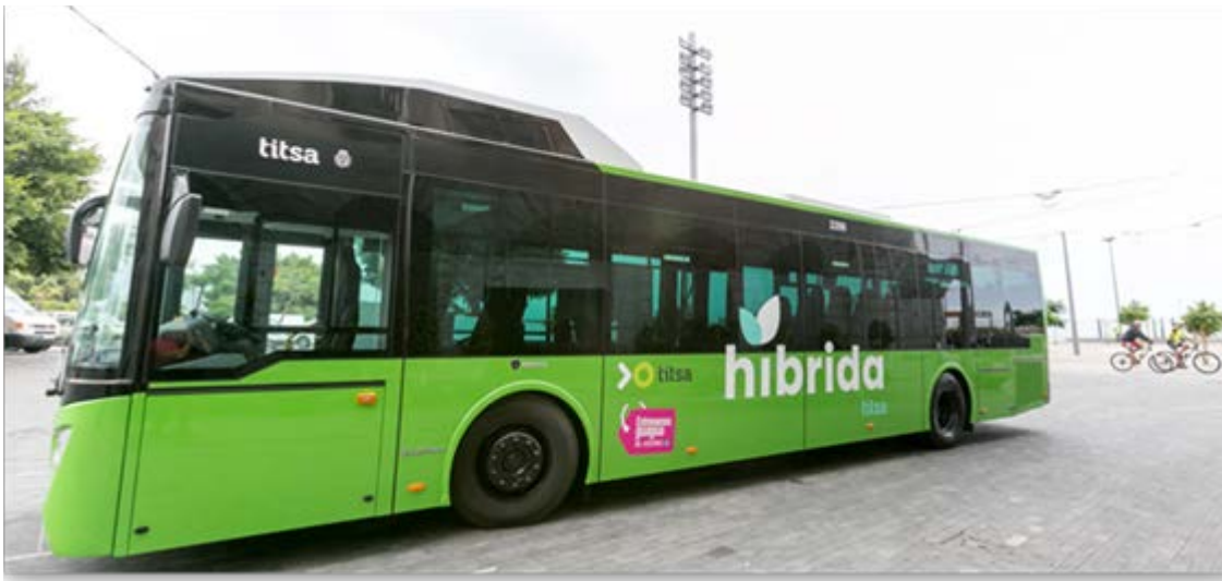
TITSA has recently acquired new hybrid buses, allowing travelling between the capital's main station and Las Teresitas beach in 100% electric mode, with an initial charge point at the central station via pantograph. Source: Marketing Area – TITSA
