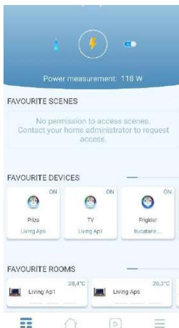
Fig. 6. Start screen shows general electricity power (118W), smart plugs (are on), room selection.
