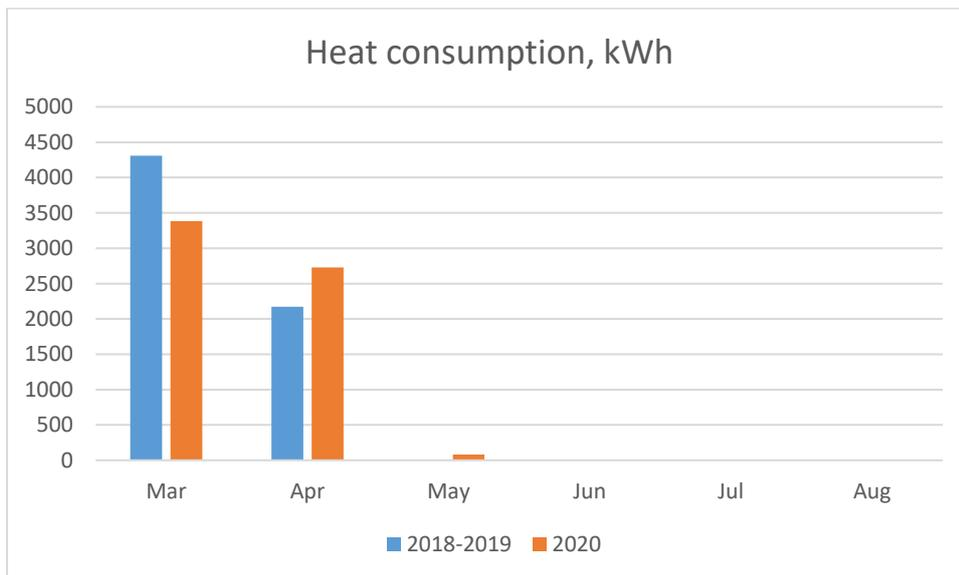
Fig.29. Monthly energy consumed for heating before and after project implementation, kWh
