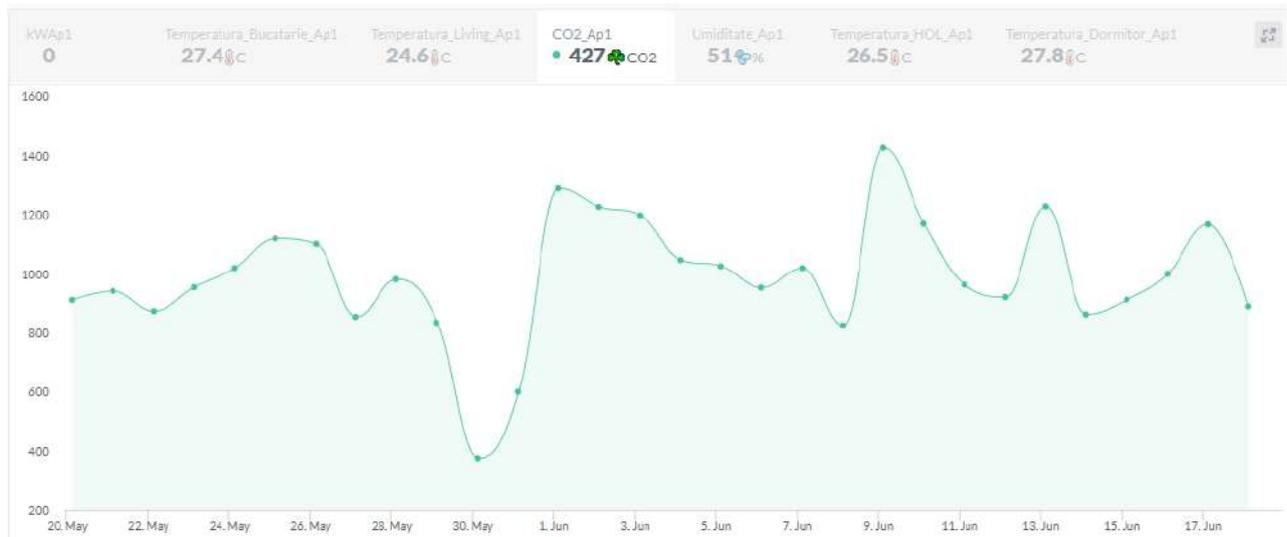
Fig. 23. One month CO2 evolution in one apartment (several days are over accepted level of max.1000ppm)
