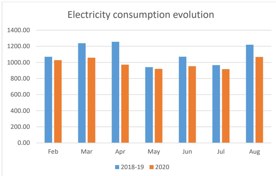
Fig.26. Monthly electricity consumption, kWh, before and after implementation, for all apartments
