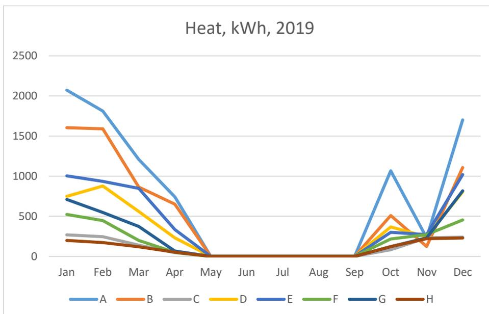
Fig 27. Monthly heat consumption, kWh, for each apartment before project implementation
