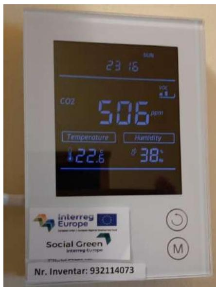
Fig. 10. Climate unit displays CO2, temperature, humidity and qualitative info for VOC
