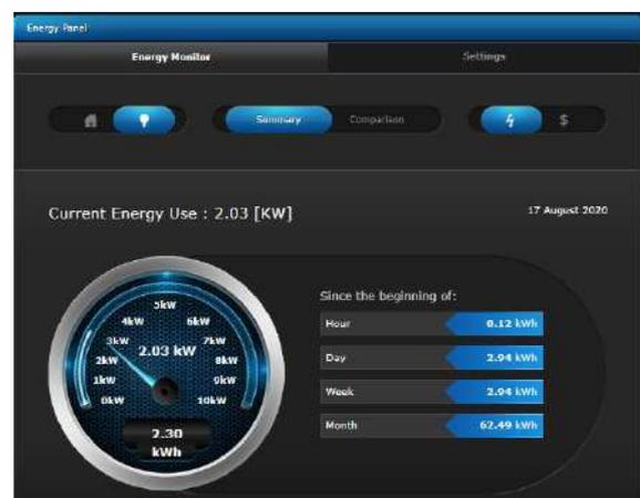
Fig.16. Energy panel shows instant power and electricity consumption (hour, day, week, month)
