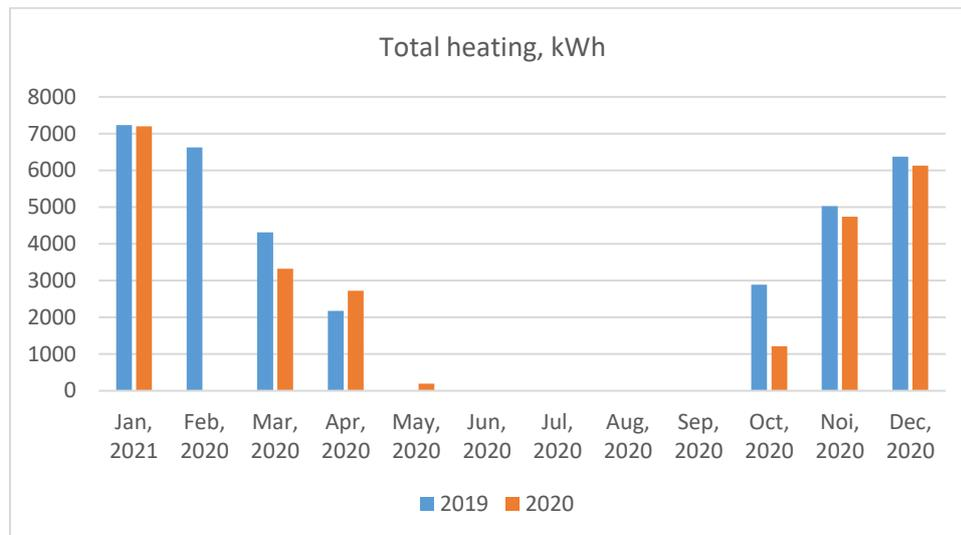
Fig.6. Monthly energy consumed for heating before and after project implementation, kWh
