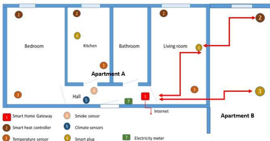
*Fig. 1. System extension using direct and repeated through smart plugs radio transmission (Zwave) to smart gateway*
