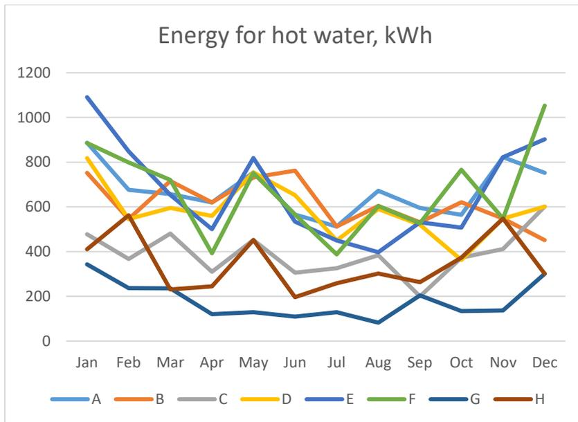
Fig.30. Monthly energy consumption of each apartment, kWh, for producing hot water
