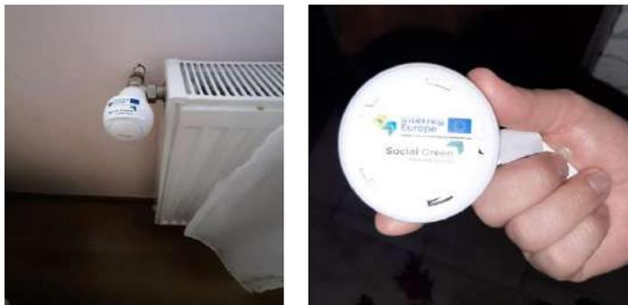
*Fig.4 – Smart Heat controller paired with temperature sensor*
