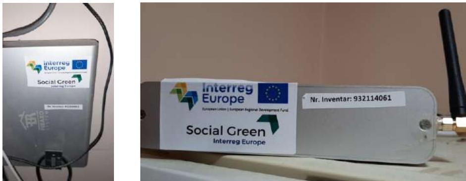
Fig.2. Smart Home Gateway – in 2 configurations, connected to internet using Ethernet cable; antenna is for Z-Wave communication with sensors
