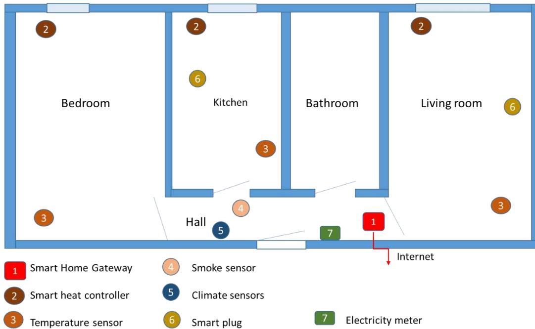
Fig. 1. System elements and their installation in apartment
