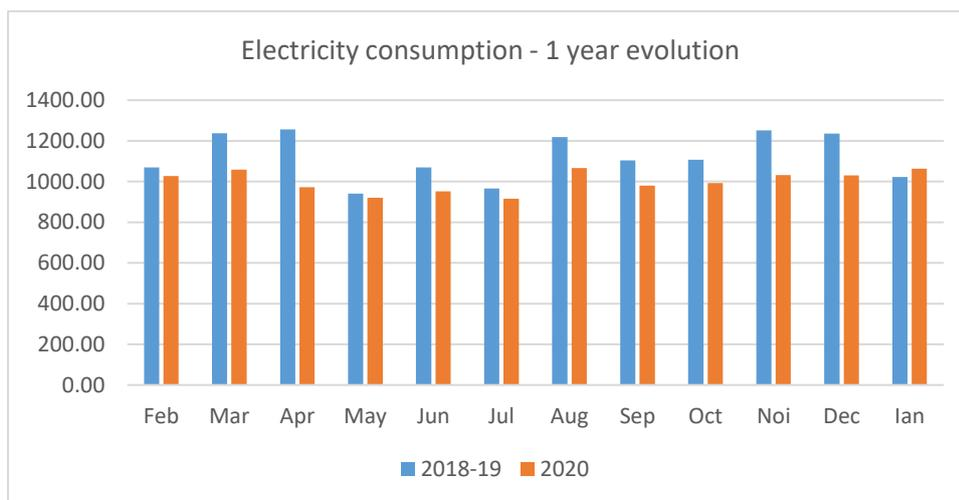
Fig.5. Comparison before and during pilot for total electricity consumption, kWh, all apartments
