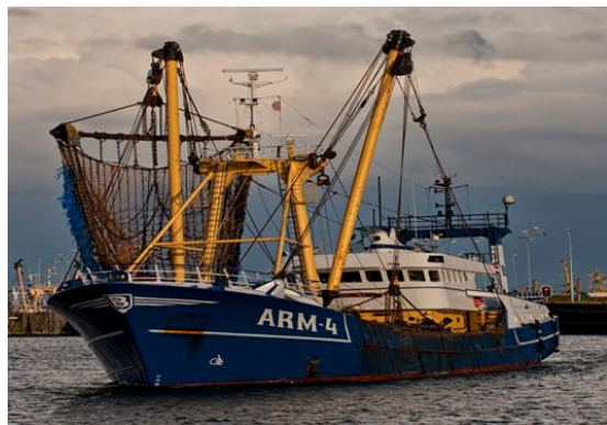
A traditional beam trawler: ARM-4, total length 45 meters (bron: Zeelandnet.nl)
