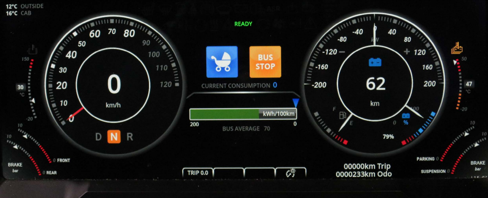
Instrumentation of a Linkker e-bus. Photo by Markku Ikonen
